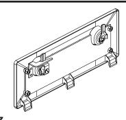
Tighten the four Nuts and turn the key to check for smooth operation.
