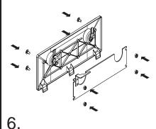
Insert the 4 Carriage Bolts from the front and mount the Stiffening Plate with the four nuts.
