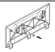
Mount the Lock Cam to the Lock. Turn the key to check the Cam turns freely. You may have to pull the Clip slightly for clearance.
