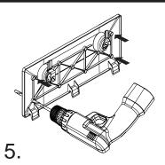
Drill four holes through the Cover using the stiffening plate as a template.
