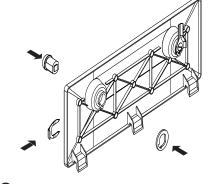
Insert the Lock from the front and the LockWasher from the rear and the Lock Clip from the side
